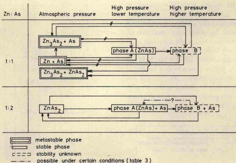
Fig. 4. Stability relationships between phases obtained from high pressures and high temperatures in the  $Zn_3As_2$ -As system.
