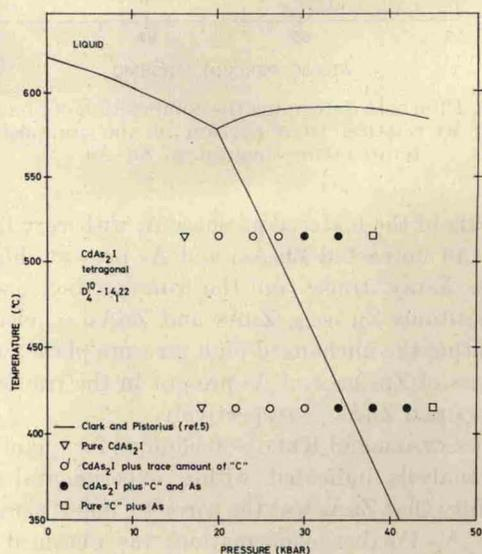
Fig. 5. Phase diagram of  $CdAs_2$ , including previously determined phase boundaries<sup>5</sup> and present results.
